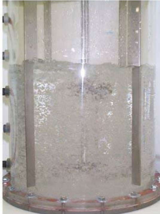
Same system with fully baffled vessel showing good gas incorporation and dispersion.
