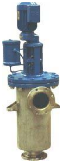
Figure 3: Gear driven mixer with double mechanical seal and lubricator pot. Mixers are also available in direct and belt driven configurations and with other shaft seals including stuffing box and single dry-running mechanical seals
