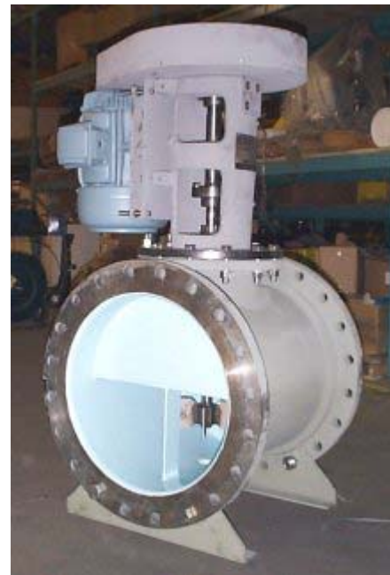
Figure 4: In-line mixer combining the two main configurations producing a staged flash mixer with a "Z" flow pattern through the vessel.
